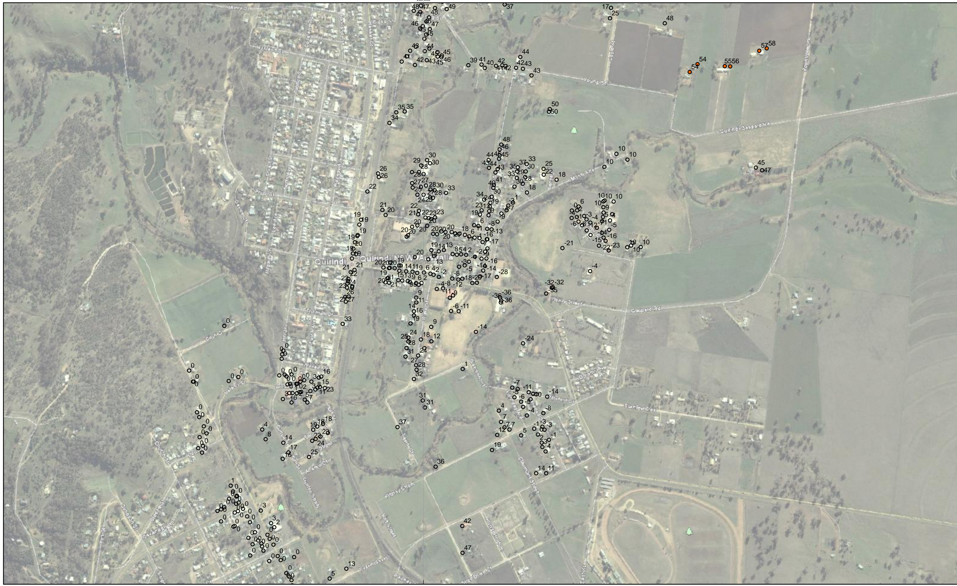
100yr ARI with 0.5m sediment along Quirindi and Jacob Joseph creeks (Flood Level Change (mm))
